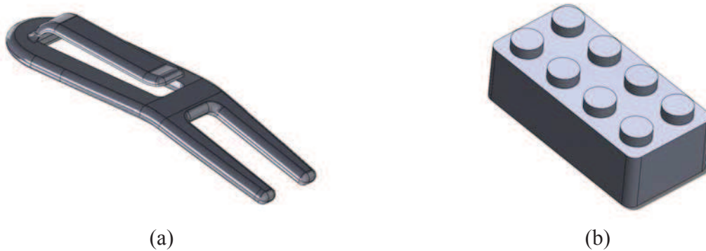
Figure 2: Examples of a part concept with a a) contoured parting line and b) a flat parting line.
