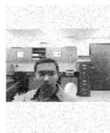
Mean filter applied to salt & pepper noise
